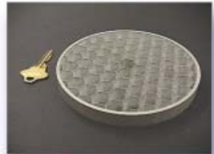
Figure 10: This photo is of a 1/2" aluminum honeycomb part with 0.025" walls. (Courtesy of www.waterjets.org (the "Waterjet Web Reference"))
