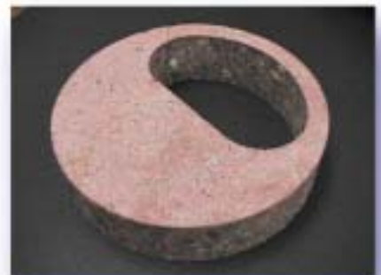
Figure 11: This photo shows 2" thick concrete (the pink color is from pigment added to the material) (Courtesy of www.waterjets.org the "Waterjet Web Reference")
